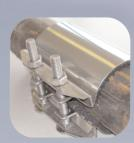
This mini clamp is as plain repair clamp. Suitable for repairing holes in small pipelines. The inside of the clamp is partially covered with a NBR or EPDM gasket. This design requires no welding and therefore no chemical treatment to passivate the clamps. Only available in predefined quantities of 100 units per position.
